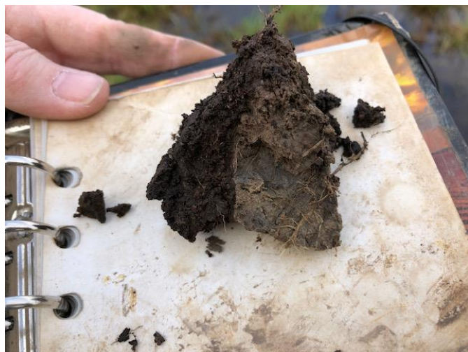
Photo 9 shows the bottom layer of the soil profile revealed at Test Plot 2. The bottom layer was a grayish brown color and no oxidized rhizospheres or redoximorphic concentrations were observed. Therefore, the hydric soil and wetland hydrology criterion are not met. Test Plot 2A conducted on April 11, 2020 and confirmed the results of Test Plot 2.
