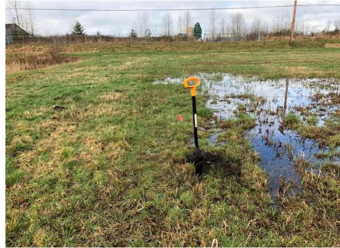
Photo 10 was taken of the area where Test Plot 3 was conducted. The area contained shallow surface water during the February 2020 field visit but was dry during the April 2020 field visit. Test Plot 3A was conducted in April and water was not present, which confirmed the non-wetland determination for this area.
